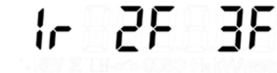
This page indicates per phase the direction of the energy. In this picture phase 1 is reverse and phase 2 and 3 are forward.
