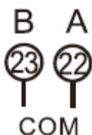
*When connecting the meter through a serial converter (RS485) for testing, please be aware that because of not implementing the complete Modbus infrastructure, there will be a need to put an additional resistor (120 ohms/ 0.25 watts) across the terminals (22 & 23) on the meter side.*
