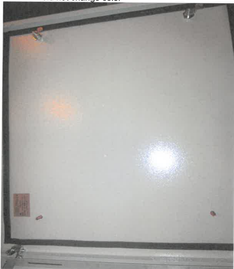
Picture 15. No water traces on the door. The control markers inside did not change color
