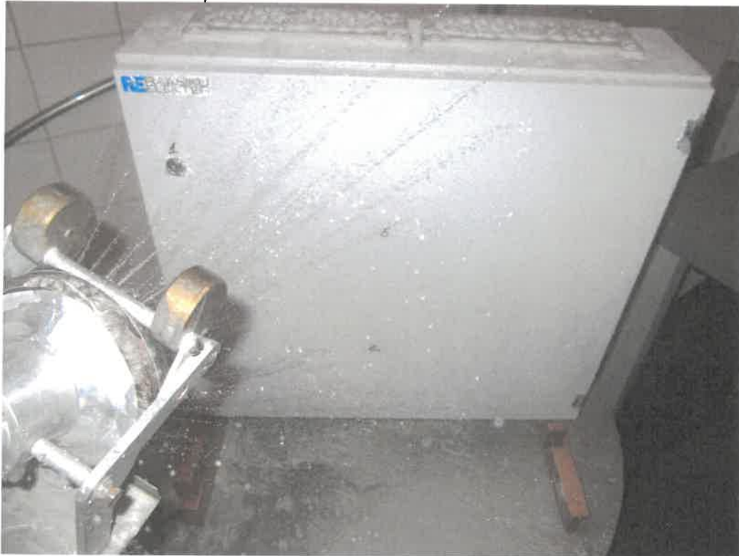
Picture 13. Test set up IPX4
