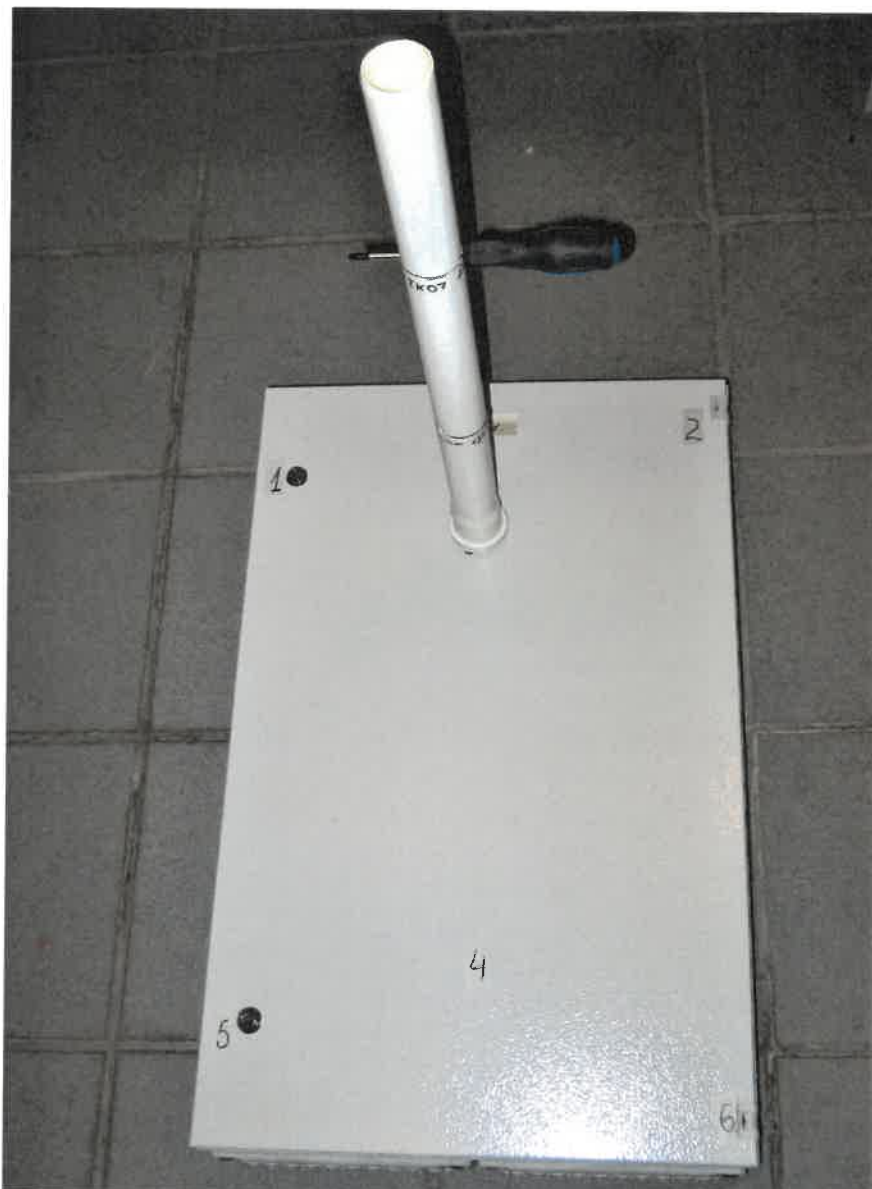
Picture 4. IK07 test set up for front of the enclosure
