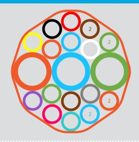
Höhle microducts are designed for long term protection of fiber optical cables. Direct Bury (DB) type of microducts are thick wall products that attain their mechanical robustness and functional performance through their intrinsic thick walls and need no further protection at underground installations.
