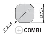
Quarter-turn cylinder lock. Universal clockwise or counter-clockwise rotation when opening / closing. Supplied with nut. Protection degree IP54.
