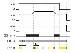
After connecting the device to the supply voltage, both LEDs on the panel will flash briefly.
