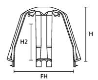
Material: Polyamide 6.6, glass-fibre reinforced
