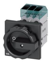
Load disconnector 3LD3, Iu 40 A Main switch 3-pole Rated operating capacity at AC-23 A at 400 V 18.5 kW Front plate mounting Basic switch with Central hole mounting 22.5mm Toggle drive black 66x66 mm
