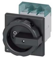
SENTRON, Switch disconnector 3LD, main switch, 3-pole, lu: 63 A, Operating power / at AC-23 A at 400 V: 22 kW, front-mounted, rotary operating mechanism, black, central mounting 22.5 mm of the handle
