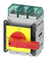
SENTRON, Switch disconnector 3LD, emergency switching-off switch, 3- pole, Iu: 160 A, operating power / at AC-23 A 400 V: 75 kW, front-mounted, knob-operated mechanism, red/yellow, 4-hole mounting of the handle
