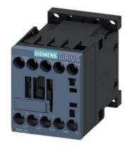
power contactor, AC-3e/AC-3, 16 A, 7.5 kW / 400 V, 3-pole, 24 V DC, auxiliary contacts: 1 NO, screw terminal, size: S00  $\,$
