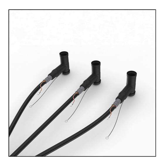
Screened separable connector for 1-core cables with Al/Cu conductor, polymeric insulation and cu-wire screen. The kit contains components for three cable cores. Mechanical lugs and all components for screen connection are included in the kit. Separable connectors are suitable for connecting cables to transformers and switchgears with bushings according to EN 50180 and EN 50181.
