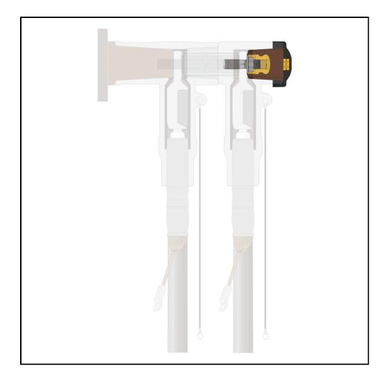
Additional insulation plug set for CONT630 screened separable connectors. The set contains components for 3 cores. Insulating plugs, threaded bolts, nuts, washers and insulating caps are included in the kit. This M16 insulation plug set enables connection of CONTB630-24Lxx series back connectors and CONT-SA10-xx series surge arresters with M12 threaded CONT630 series separable connectors.
