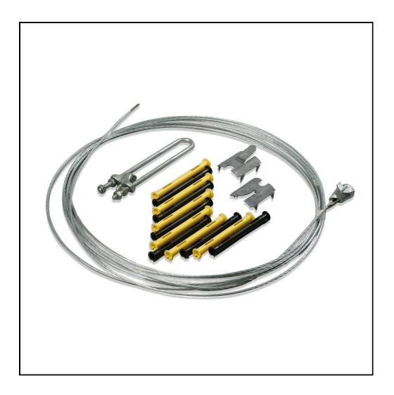
An uninsulated set for low voltage lines. The wire gauge is 25 mm² steel wire and the permitted load is up to 17.5 kN. All steel parts are hot-dip galvanized and plastic marking tubes are of weather and UV-resistant material.
