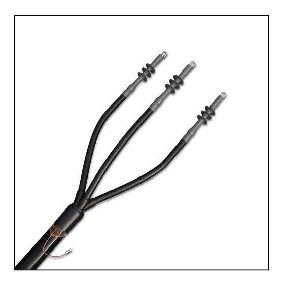
Hybrid indoor termination for 3-core cables with Al/Cu conductor, polymeric insulation and Cuwire screen. Mechanical lugs for conductor and screen wire connection are included in the kit. The termination kits include cold shrinkable termination bodies with integrated stress control elements, heat shrinkable semi-conducting breakout and semi-conducting core protection tubes and all the additional components needed for assembly.
