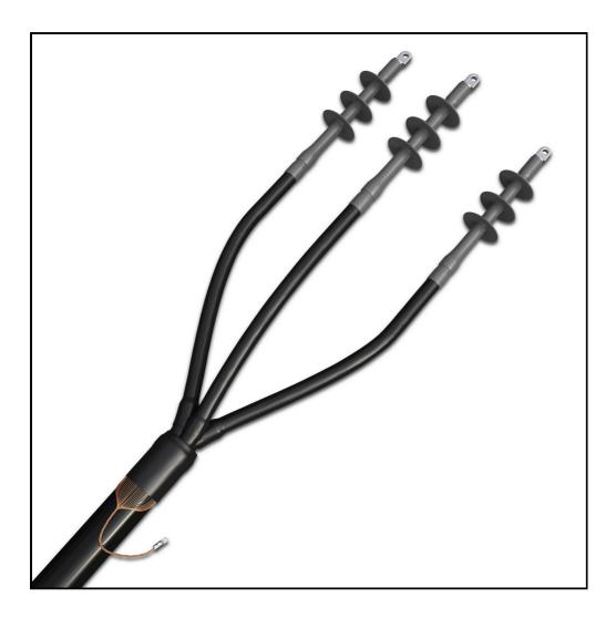
Hybrid outdoor termination for 3-core cables with Al/Cu conductor, polymeric insulation and Cuwire screen. Mechanical lugs for conductor and screen wire connection are included in the kit. The termination kits include cold shrinkable termination bodies with integrated stress control elements, heat shrinkable semi-conducting breakout and semi-conducting core protection tubes and all the additional components needed for assembly.
