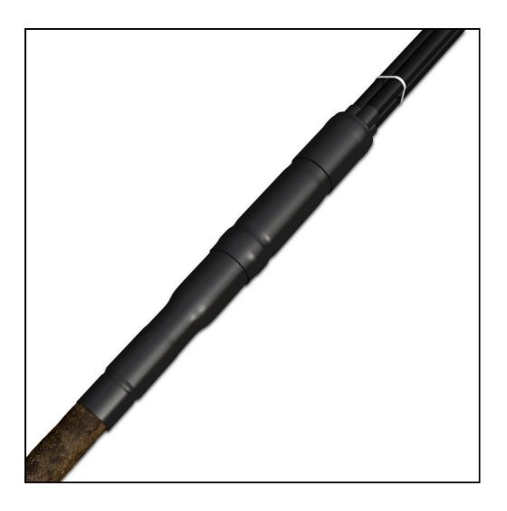
The joint kit is used for jointing of max. 12 kV three core cables with belted paper insulation and lead or aluminium sheath, either armoured or non-armoured, to single core cables with XLPE insulation and copper wire or tape shield. The kit includes the shear head bolt cable connectors suitable both for aluminium and copper conductors, and all the components needed for jointing.
