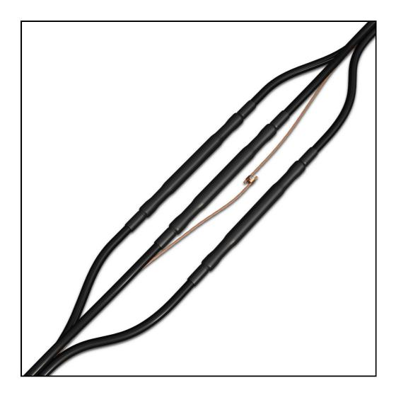
Cold shrink hybrid joint for 1-core cables with Al/Cu conductor, polymeric insulation and Allaminate screen. The kit contains components for three cable cores. Mechanical connectors are included in the kit. Hybrid joint kits include cold shrinkable joint bodies with integrated geometric stress control elements, tubular copper braids for screen connection, heat shrinkable outer jacket tubes and all the additional components needed for jointing.
