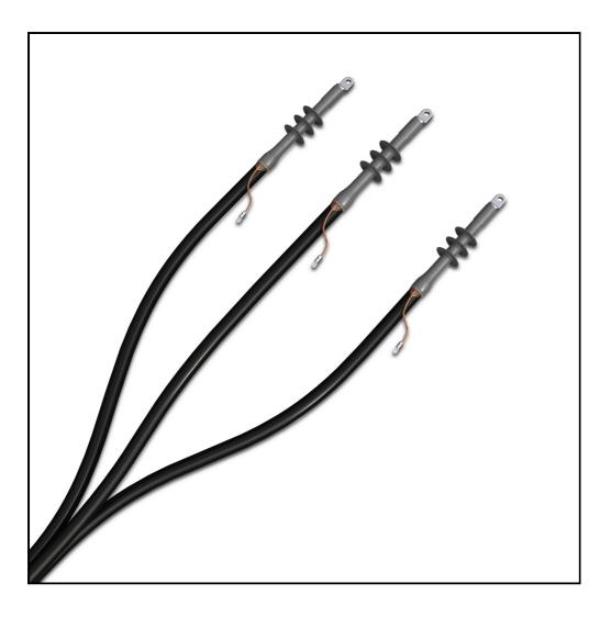
Cold shrink indoor termination for 1-core cables with Al/Cu conductor, polymeric insulation and Cu-wire screen. The kit contains components for three cable cores. Mechanical lugs for conductor and screen wire connection are included in the kit. The termination kits include cold shrinkable termination bodies with integrated geometric stress control elements and all the additional components needed for assembly.
