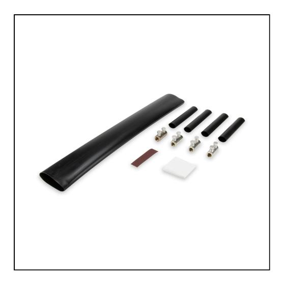
The joint kit is used for jointing 1 kV cables with plastic insulation and plastic outer sheath. The kit is suitable for 4 to 4 core and 4 to 3+1 core cables. The kit includes four screw connectors suitable both for aluminium and copper conductors, grinding and cleaning materials, four heat shrink tubes for insulation and one for outer protection.
