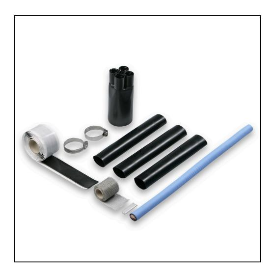
The additional kit is used together with the 1 kV joint kit SJK for jointing of belted paper insulated, aluminium sheathed 3 core cables (e.g. APAKM). The kit is suitable for transition from paper insulated cable to plastic insulated. The kit includes three heat shrink tubes for protection of the paper insulation, a heat shrink breakout, a piece of H07V-K cable for jointing the aluminium sheaths.
