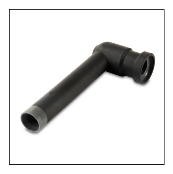
Screened 250A elbow type straight connectors are used for connections to transformers and switchgears up to 24kV with bushings according to EN 50180 and EN 50181, connection type A (250 A). Suitable for 3-core plastic cables (XLPE, EPR, PE, etc.) both indoors and outdoors. Three phase set including shear head bolt cable lugs.
