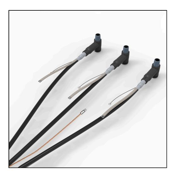
Screened separable back connector for 1-core cables with Al/Cu conductor, polymeric insulation and Al-laminate screen. The kit contains components for three cable cores. Mechanical lugs and all components for screen connection are included in the kit. CONTB630-24 series separable back connectors are suitable for connecting cables in parallel with CONT630-24 series T-connectors.
