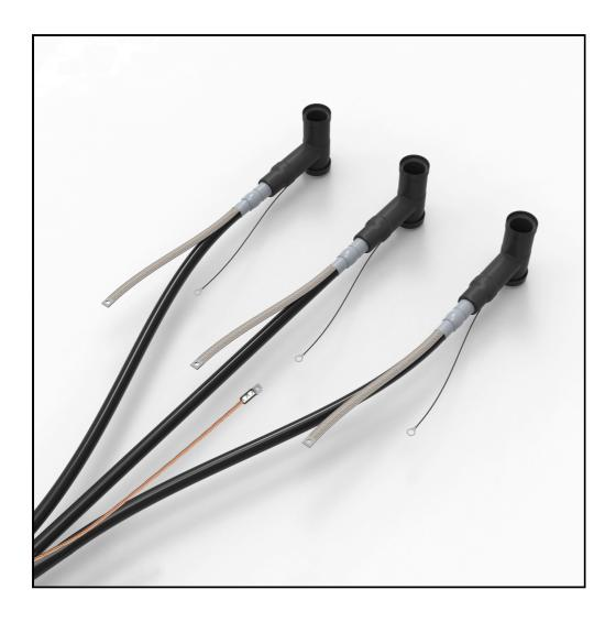
Screened separable connector for 1-core cables with Al/Cu conductor, polymeric insulation and Allaminate screen. The kit contains components for three cable cores. Mechanical lugs and all components for screen connection are included in the kit. Separable connectors are suitable for connecting cables to transformers and switchgears with bushings according to EN 50180 and EN 50181.
