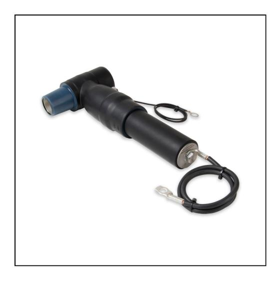
The screened surge arrester can be connected to CONT630 and CONTB630 connectors. The arrester protects transformers, switchgears and transmission lines against atmospheric and switching over voltages. Set includes three pcs of surge arresters and connection bolt.
