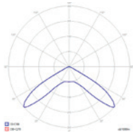
SQ - niskie strefy otwarte / square beam open spaces optics
