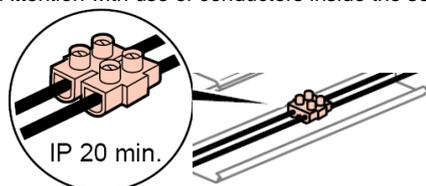
Inside the mini-trunkings, connection of the conductors using "domino" to respect the IP 20 mini.
