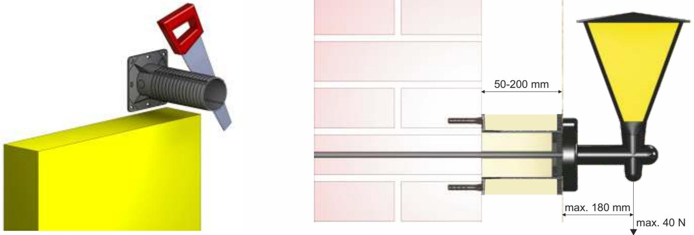
There is necessary to cut the carrier including inserted insulation before installation depending on layer thickness insulation.
